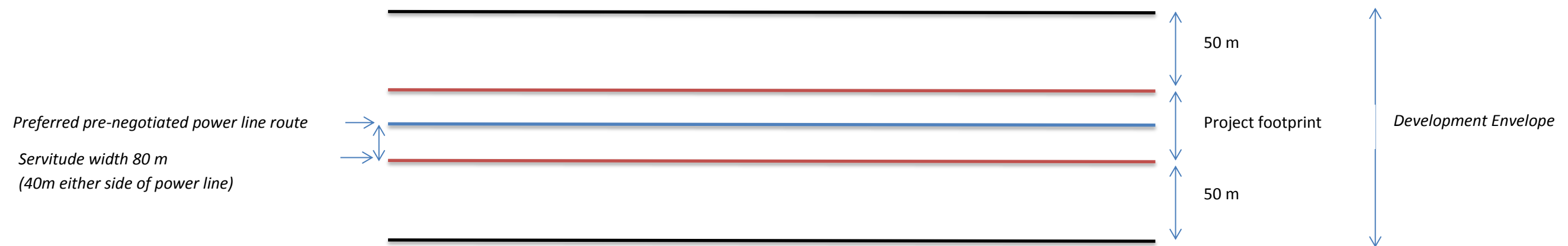
Figure 4: Route profile in context of servitude and Development Envelope for typical 765kV power line
